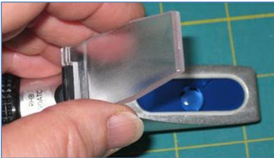
Step 1: Lift the plastic cover and place a droplet of honey on the refractometer.
